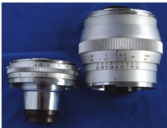
This comparison of a Distagon 2,8/25 (right) with a Biogon 4,5/21 (left), both mounted for the Contarex from Zeiss Ikon, demonstrates once again the great differences in the two designs. The Biogon is nearly as long, but disappears for the most part into the camera; this of course brings its mirror to rest.
